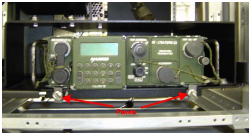
Figure 3 – Radio Mount pawls
