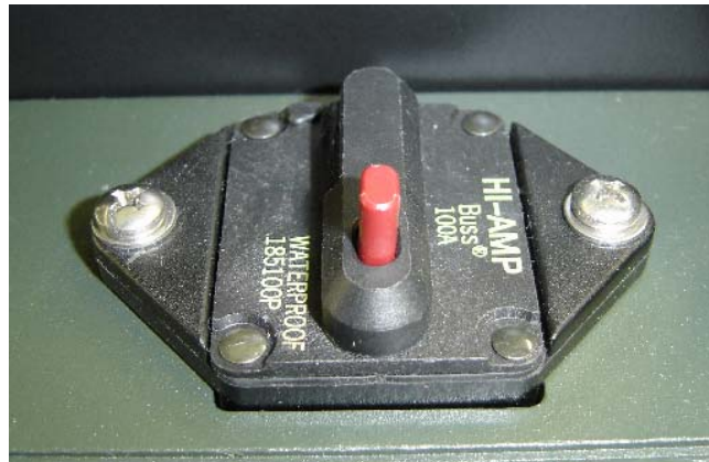
Figure 8 – Circuit Breaker in ON position
