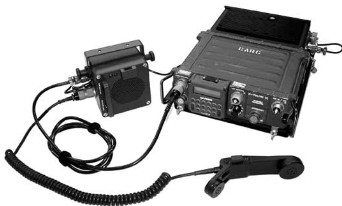
FIGURE 1-2 MRC-93 ATTACHED TO AN/PRC-117F, THE RMT-2 MOUNT AND MRC-67 AMPLIFIED SPEAKER
