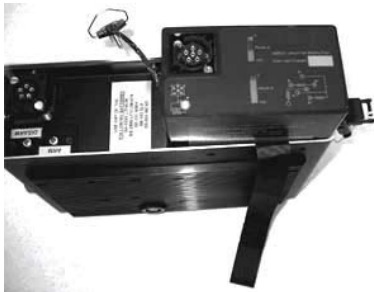
Figure 2-2 BATTERY AND STRAP
