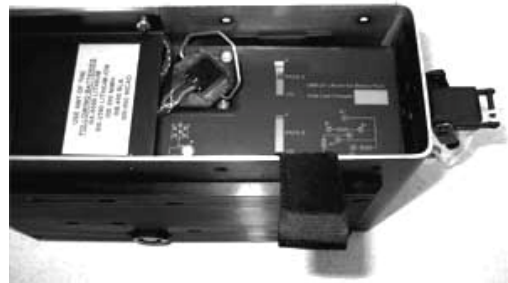
Figure 2-3 BATTERY IN POSITION WITH CABLE
