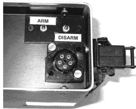
FIGURE 2-3 BATTERY CONNECTOR AND ARM/DISARM SWITCHES
